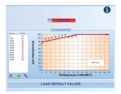
To correctly use and configure this functionality, the depreciation curve of the LED module lumen output to be supplied must be known. This curve can differ for the different LED modules on the market and depends on both the operating point and the thermal conditions under which it is working.
