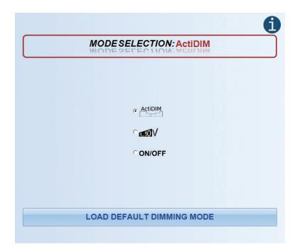
The iLC CORE control gear is able to select the most suitable dimming method for each application. The choice of a specific dimming mode activates its configuration parameters and deactivates other dimming methods.
