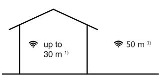
eBLUE uses mesh network technology, i.e. each eBLUE 0-10V / DALI acts also as a repeater. Much longer ranges can be achieved by using multiple eBLUEs 0-10V / DALI.
