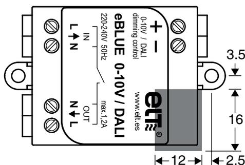
Picture 2. Suggested minimum antenna cut-out
