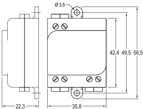
Wireless control device for LED, FLUO, HID and halogen control gears with 0-10V, 1-10V or DALI dimming interface. The control output can be configured either as analog 0-10V (1-10V) or digital stand-alone DALI control interface.
