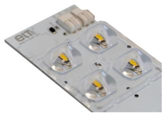
Individual lenses are used for street lighting, as they are highly efficient, made of plastic and in some cases protected by means of a flat glass. They offer asymmetric roadway photometry that directs the light to specific areas to avoid light loss.
