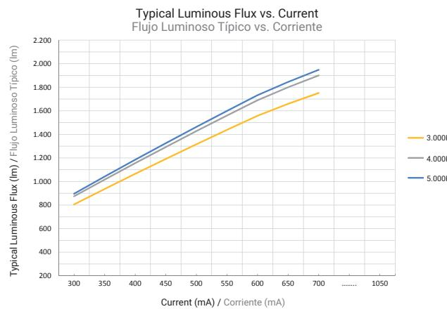
\* Luminous flux tolerance  $\pm 10\%$  and for colour temperature  $\pm 7\%$  guaranteeing a standard deviation of  $\pm 3\%$  per module eLED
