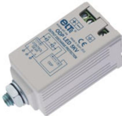
When a high electrostatic charge storage exists between the LED module and the luminaire, the ODP protection circuit gets rid off that charge safely through Earth, avoiding that discharge to go across the LED, producing permanent damages in the load.
