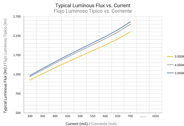
\* Luminous flux tolerance ±10% and for colour temperature ±7% guaranteeing a standard deviation of ±3 % per module eLED
